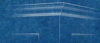
CHAIR RAIL: 1X5 S4S VERTICAL, 1X6 TOP RAIL, 2440 HEADER, NOSING-POP LEDGE
