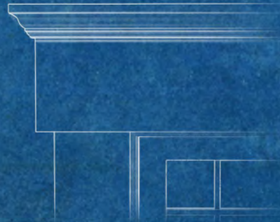
CASING: 5/4X8 S4S WITH 01435 HEADER
